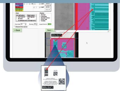
The LVS-7500 label inspection system provides 100% label inspection as labels are printed at production printing speeds. In the event of a label defect the printer is automatically stop ensuring that the defective label is confirmed by an operator and removed.
